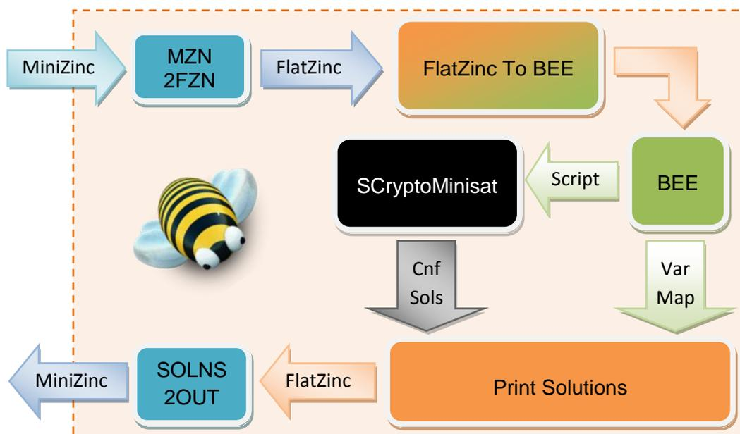
These components are written in different languages (such as Prolog, Python, and C++) and implemented as individual black boxes. The components are "glued" together using. The black box components include: MZN2FZN & SOLNS2OUT (Blue in the figure) , *BEE* (Green in the figure), and SCryptoMinisat (Black in the figure) .
